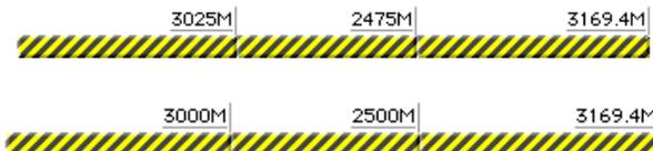
Figure 2.3: Reducing the size of the first partition from 53 Mbytes to 50 Mbytes increases the size of the second partition from 27 Mbytes to 30 Mbytes. Yellow striped areas indicate that data will be destroyed when the new partitions are installed.
